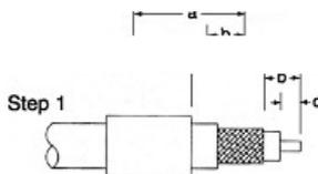
**Step 1** Strip cable jacket, braid, and dielectric to dimensions shown. All cuts are to be sharp and square.
