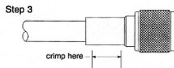
**Step 3** Install cable assembly into body assembly so inner ferrule portion slides under braid. Push cable assembly forward until contact snaps into place in insulator. Slide outer ferrule over braid and up against connector body. Crimp outer ferrule using crimp tool
